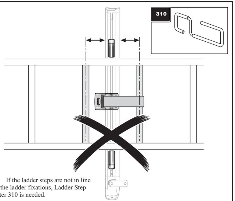
**GB** If the ladder steps are not in line with the ladder fixations, Ladder Step adapter 310 is needed.
